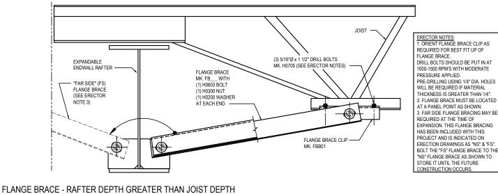
ALL FLANGE BRACE CONNECTIONS REQUIRE 1/2" x 2" A325 BOLTS UNLESS NOTED OTHERWISE SEE PLANS AND ELEVATIONS FOR FLANGE BRACE LOCATIONS, PART MARKS & QUANTITIES
