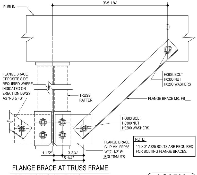
BOLTED FLANGE BRACING AT 6" FLANGES SEE PLANS AND ELEVATIONS FOR FLANGE BRACE PART MARKS AG0500
