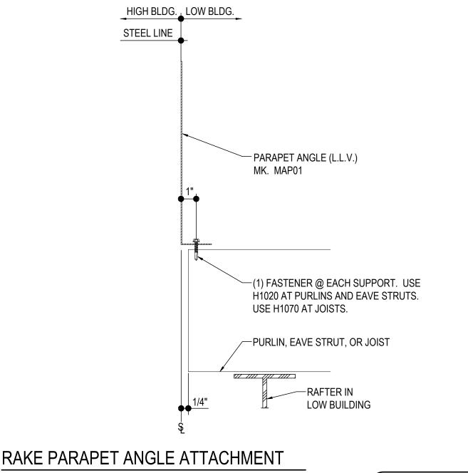
RAKE PARAPET (RAFTER IN LOW BUILDING)
