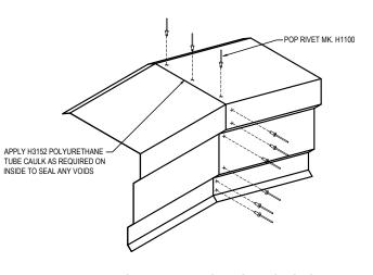
FIELD FABRICATED PEAK BOX INSTRUCTIONS REFERENCE PEAK BOX DETAIL FOR INSTALLATION
