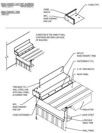
NOTE: ALL POP RIVETS AND FASTENERS ARE TO BE SET "IN" THE MASTIC OR CAULK
