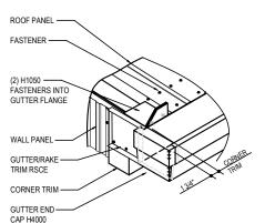
APPLY TUBE CAULK TO 3 SIDES OF THE RAKE CAP
