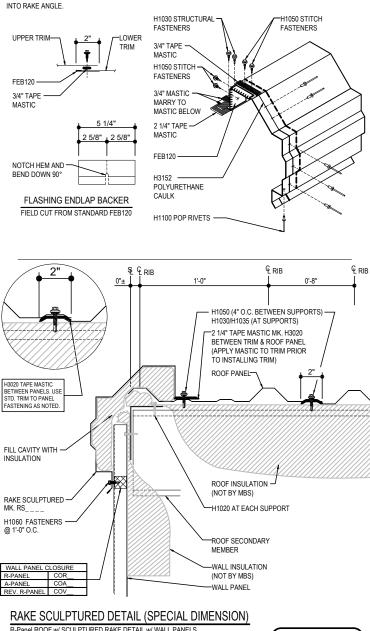
R-Panel ROOF w/ SCULPTURED RAKE DETAIL w/ WALL PANELS SEE WALL SHEETING ERECTION NOTES FOR WALL PANEL FASTENER LOCATIONS DE0015
