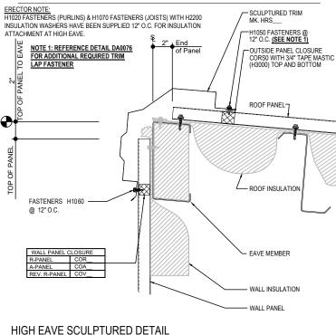
HIGH EAVE SCULPTURED DETAIL w/ R-Panel ROOF & WALL PANELS SEE WALL SHEETING ERECTION NOTES FOR WALL PANEL FASTENER LOCATIONS
