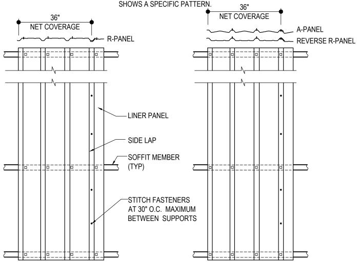
SOFFIT PANEL ERECTION DETAIL
