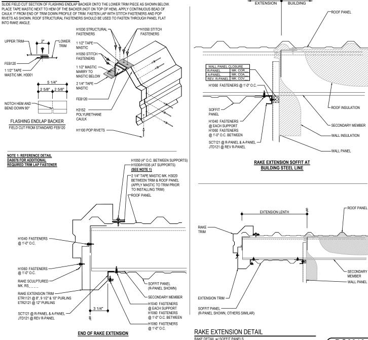
RAKE DETAIL W/ SOFFIT PANELS SEE WALL SHEETING ERECTION NOTES FOR WALL PANEL FASTENER LOCATIONS
