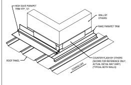
HIGH EAVE PARAPET- LOW EXTENDS DETAIL SHOWN WITH ROOF PANEL, WALL PANEL, AND CORNER TRI MASONRY AND INSULATED WALL PANEL CONDITIONS SIMILAR.
