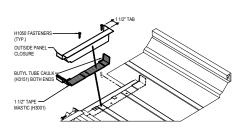
BEFORE INSTALLING THE HIGH EAVE PARAPET TRIM (HTP\_121), PLACE TAPE MASTIC AND CAULK ALONG THE FULL LENGTH OF THE TOP LEG OF THE OUTSIDE PANEL CLOSURES AS INDICATED IN THE BASIC INSTALLATION DETAIL AND BELOW.
