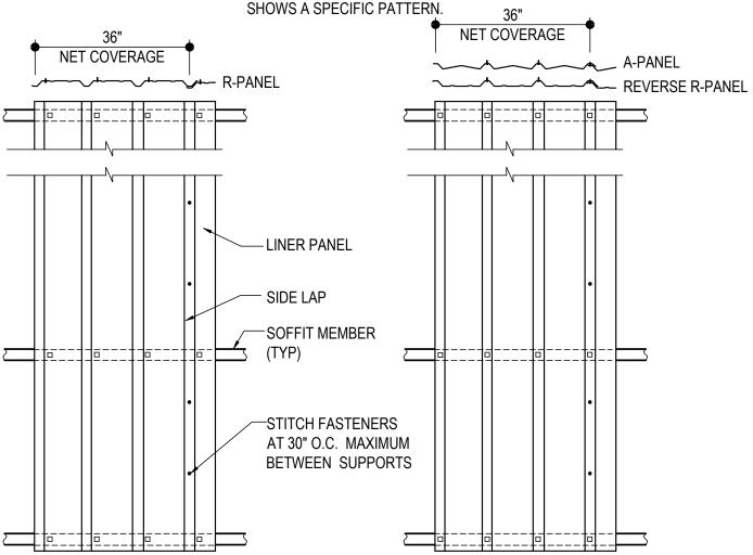
SOFFIT PANEL ERECTION DETAIL
