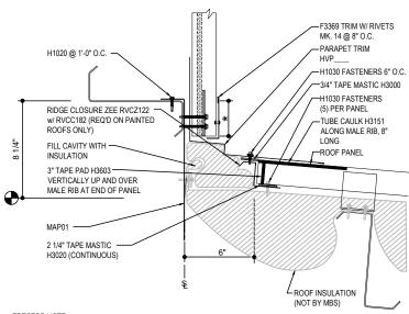
ERECTOR NOTE: INSULATION TIE-OFF SHOWN IS ONE METHOD. MAY REQUIRE DIFFERENT METHOD BASED ON SEQUENCE.H1020 FASTENERS (PURLINS) & H1070 FASTENERS (JOISTS) WITH H2200 INSULATION WASHERS HAVE BEEN SUPPLIED 12" O.C. FOR INSULATION ATTACHMENT
