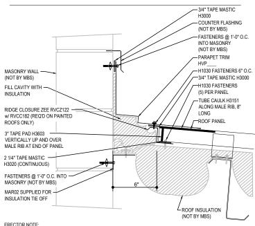
ERECTOR NOTE: INSULATION TIE-OFF SHOWN IS ONE METHOD. MAY REQUIRE DIFFERENT METHOD BASED ON SEQUENCE H1020 FASTENERS (PURLINS) & H1070 FASTENERS (JOISTS) WITH H2200 INSULATION WASHERS HAVE BEEN SUPPLIED 12" O.C. FOR INSULATION ATTACHMENT
