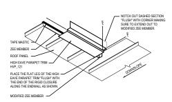
SIEP 4: BEFORE INSTALLING THE RAKE PARAPET TRIM (RPU121), PLACE TAPE MASTIC ON TOP OF THE ROOF PANEL, FROM THE LOW END OF THE RAKE PARAPET TRIM TO THE HIGH END OF THE PANEL (DO NOT REMOVE THE PAPER BACK FROM THE MASTIC UNIT. THE TASIS IN THE RAKE PARAPET TRIM ARE CREATED).
