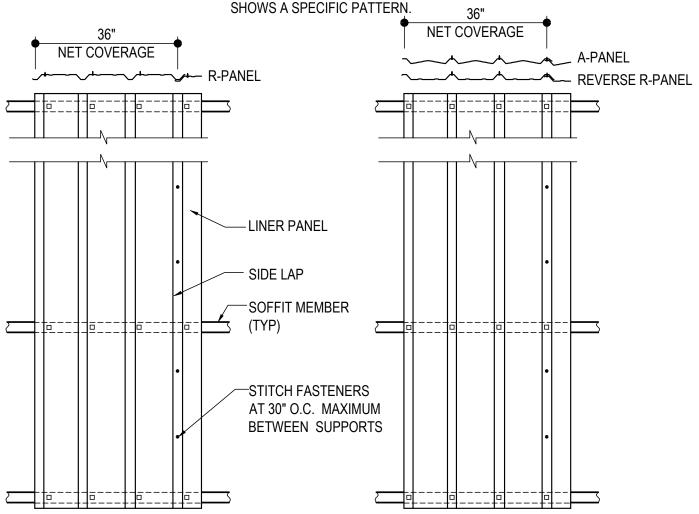
SOFFIT PANEL ERECTION DETAIL
