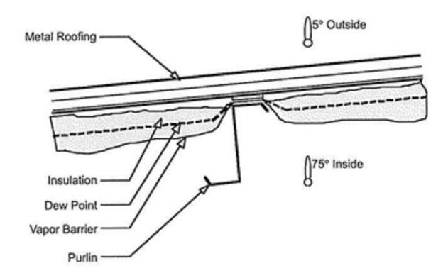
Inspect the exterior of your building for exposed insulation and call your contractor immediately if found. Exposed insulation will wick and hold water against the ends and back side of the panels, causing rust to occur.
