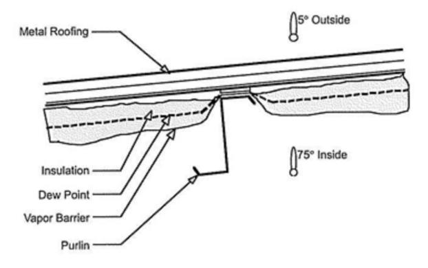
Inspect the exterior of your building for exposed insulation and call your contractor immediately if found. Exposed insulation will wick and hold water against the ends and back side of the panels, causing rust to occur.
