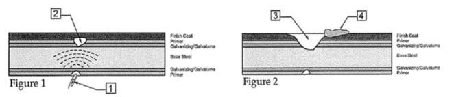
Figure 1 1. Hot sparks caused from cutting the panel burns through the primer. 2. The primer under the finish coat on the opposite side is also burned.
